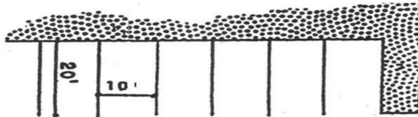
FIGURE D - 90° PARKING MANEUVERING LANE = 17 FT MINIMUM
