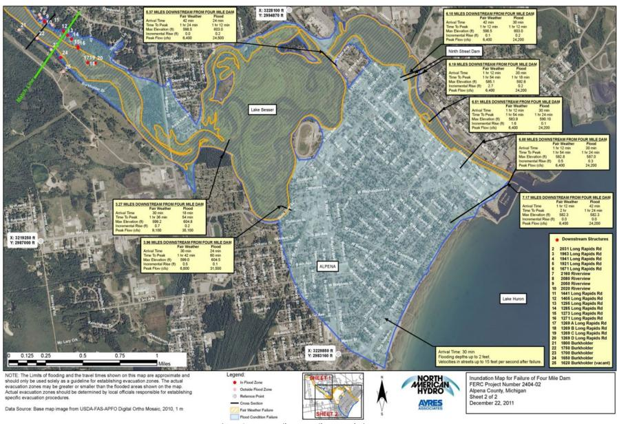
Figure 6-14 Four Mile Dam Failure Inundation Map
