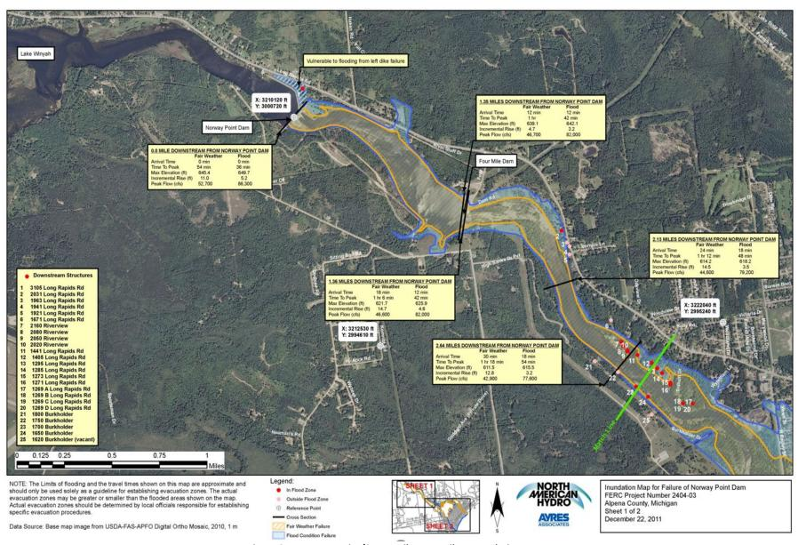
Figure 6-15 Norway Point/Seven Mile Dam Failure Inundation Map
