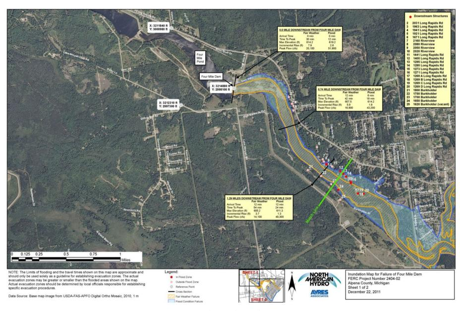
Figure 6-13 Four Mile Dam Failure Inundation Map
