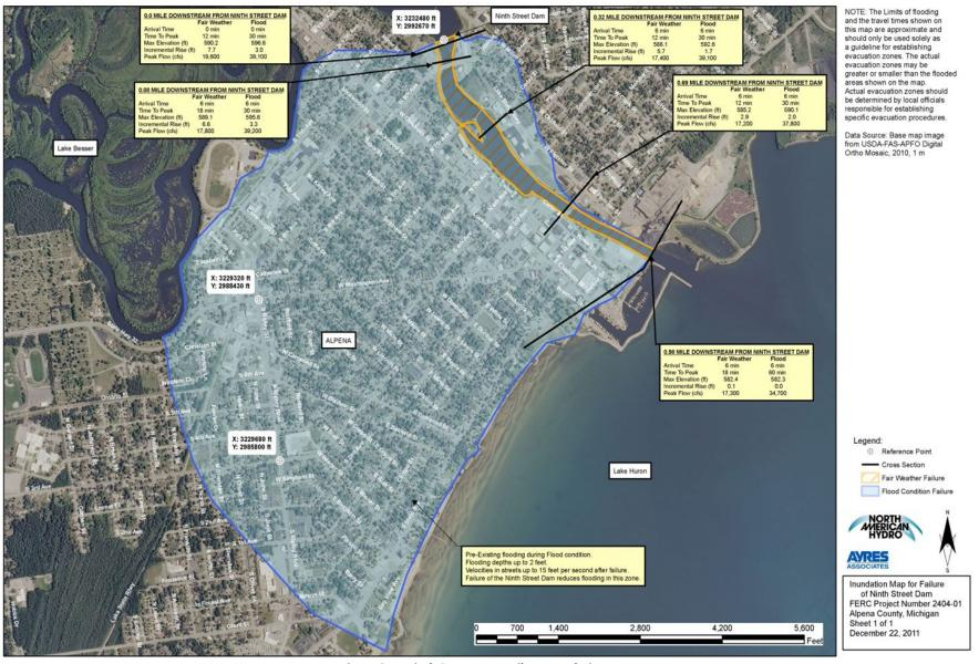
Figure 6-17 Ninth Street Dam Failure Inundation Map
