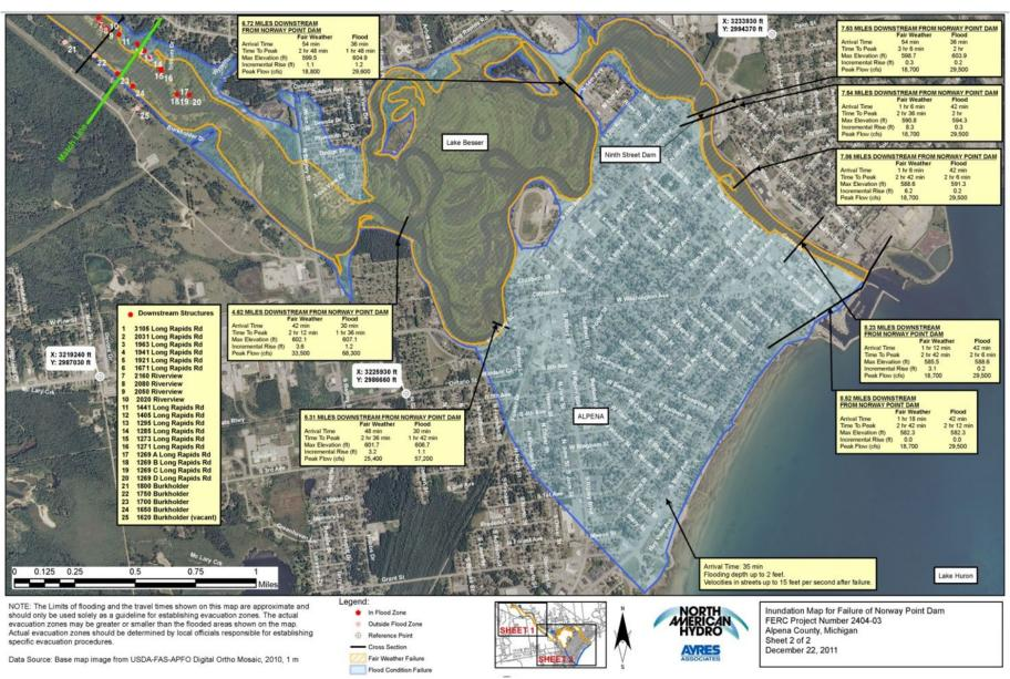
Figure 6-16 Norway Point/Seven Mile Dam Failure Inundation Map
