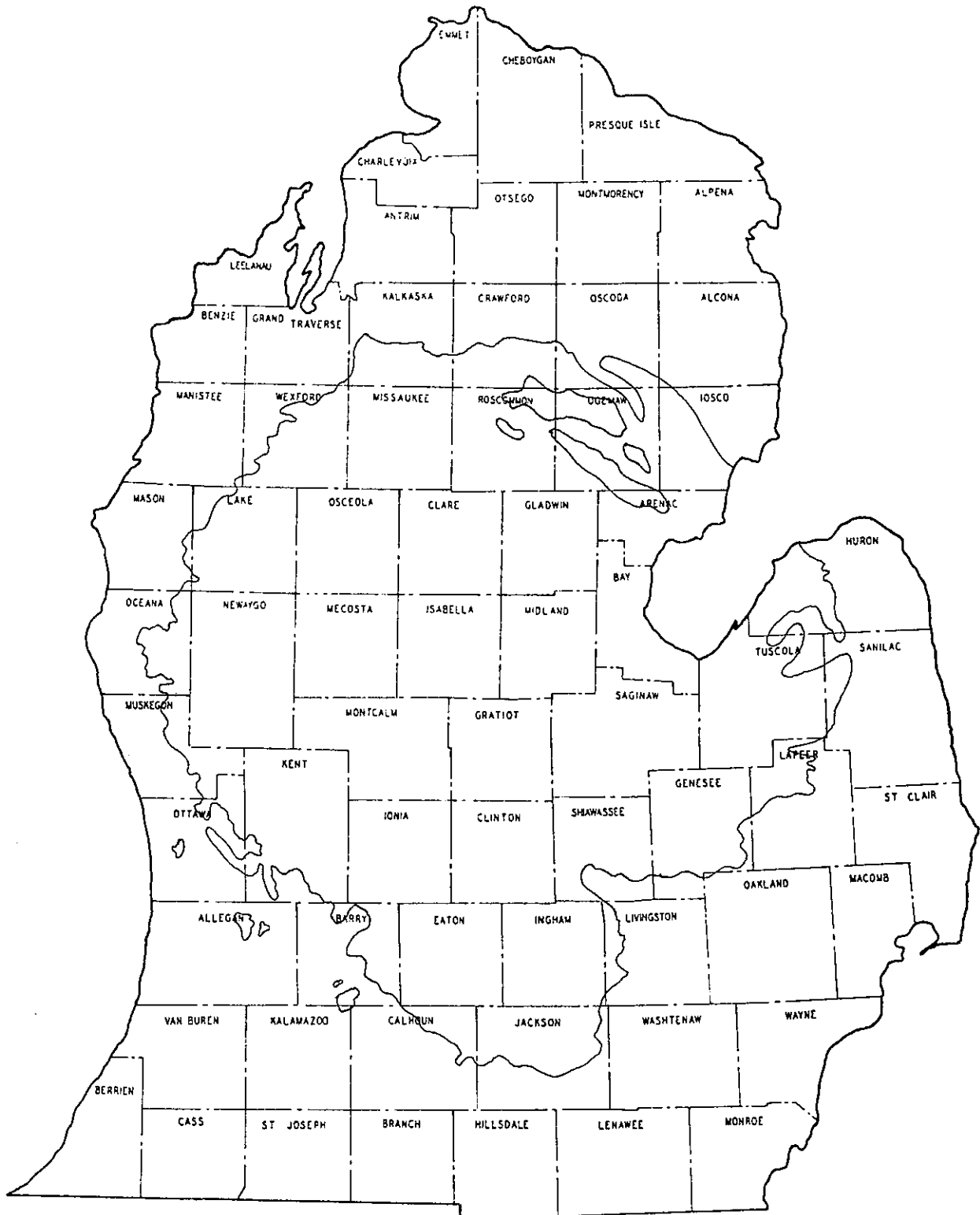
Figure 2: Map of southern Michigan showing extent of Michigan Formation beneath glacial drift. Outline is the zero thickness line where the formation pinches out from its thickest section in about the center of Missaukee County.
