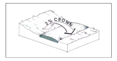
FIGURE 4-10: TRAIL WITH DRAINAGE SWALE
