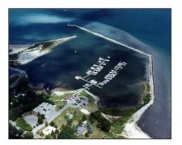
The Harrisville Harbor was completed by the US Army Corps of Engineers in 1961. A large basin had to be created along the shoreline by dynamite, dredging, and removing large boulders. The limestone wall was constructed to create the harbor of refuge for anchorage and shelter. A fixed dock was built in 1963,
