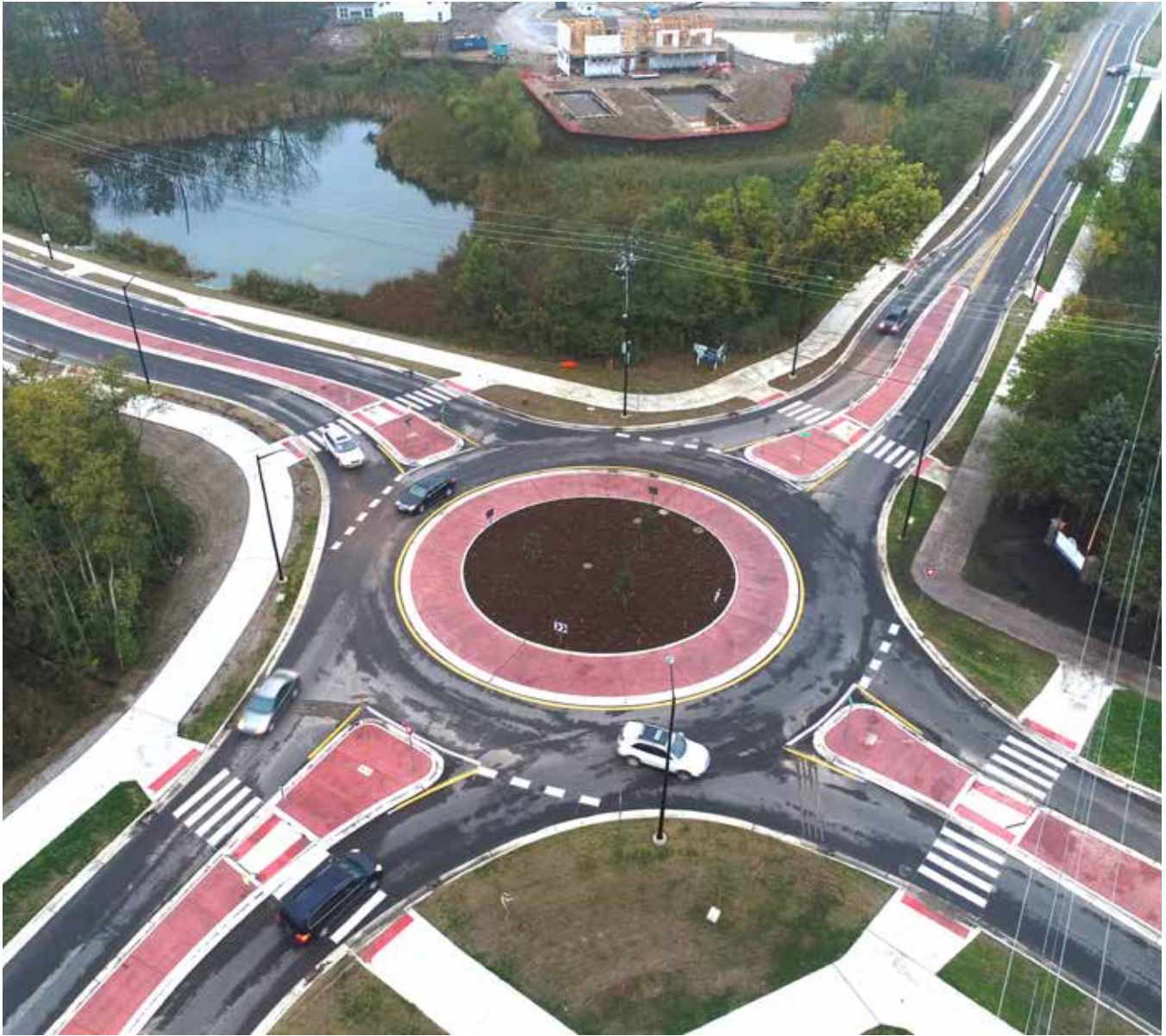
Roundabouts can vastly improve traffic flow and safety conditions at complicated intersections.
