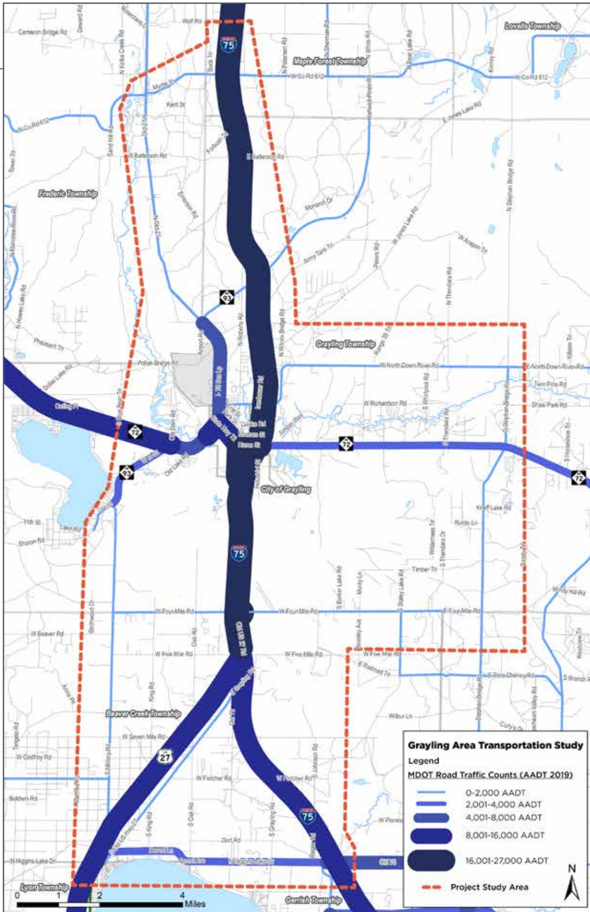
FIGURE 13: MDOT Roadway Traffic Counts (AADT 2019)
