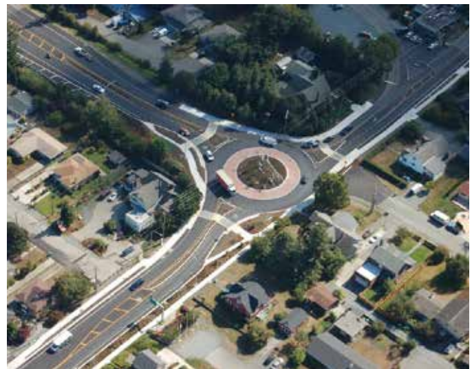
Roundabouts remove the traffic signal and allow for traffic to move continuously through an intersection.
