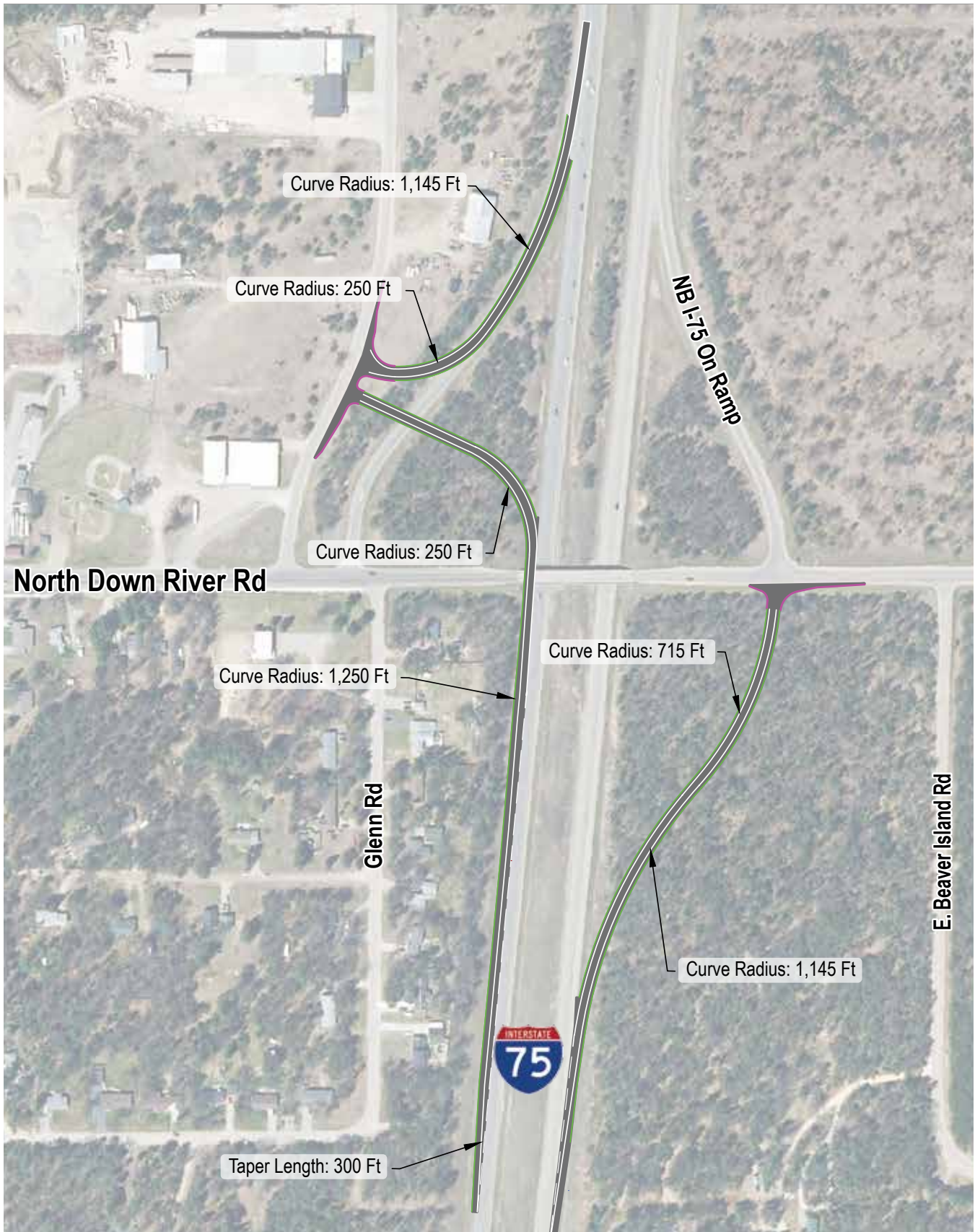
FIGURE 19: Detailed N. Down River Road Interchange Improvements
