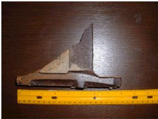
Figure 5.7. Fragments of cast iron reflector mounts are sometimes found in the roadway.
