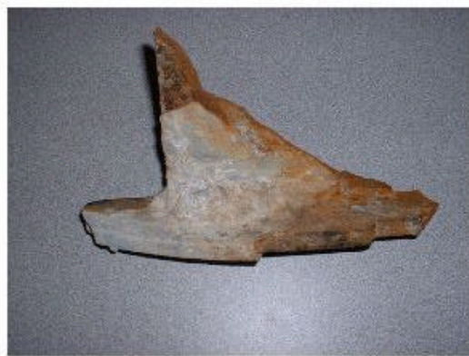
Figure 5.7. Fragments of cast iron reflector mounts are sometimes found in the roadway.
